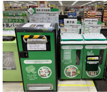
Special collection box with compression function
